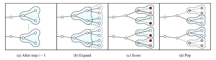
Figure 3: Sequential decoding process using the bubble decoder with B=2, d=2, k=1. (a) At the beginning of step i, the partial trees have depth d-1. (b) Grow them out to depth d. (c) Propagate the smallest path costs back through the tree. (d) Select the B best children, pruning the rest. Advance to the next step and repeat.
