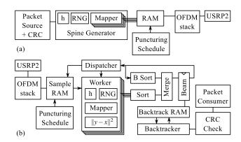
Figure 5: Hardware implementation block diagram, showing the spinal transmitter (a) and receiver (b).
