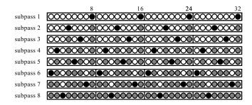
Figure 4: Puncturing schedule. In each subpass, the sender transmits symbols for spine values marked by dark circles; shaded circles represent spine values that have already been sent in a previous subpass.
