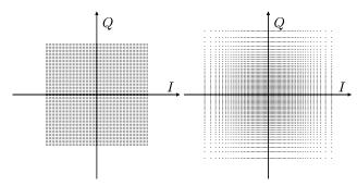
Figure 2: Uniform (left) and truncated Gaussian (right) constellation mapping functions. Same average power; c=6; truncated Gaussian with  $\beta=2$ .
