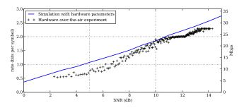
Figure 9: Rates achieved by the hardware over-the-air experiment, compared to a software simulation with similar parameters. Throughput (right axis) shows equivalent link rate for a 20 MHz 802.11a/g channel.
