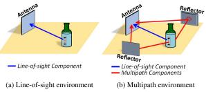
Figure 3: Typical Ray-Tracing Channel Approximations.
