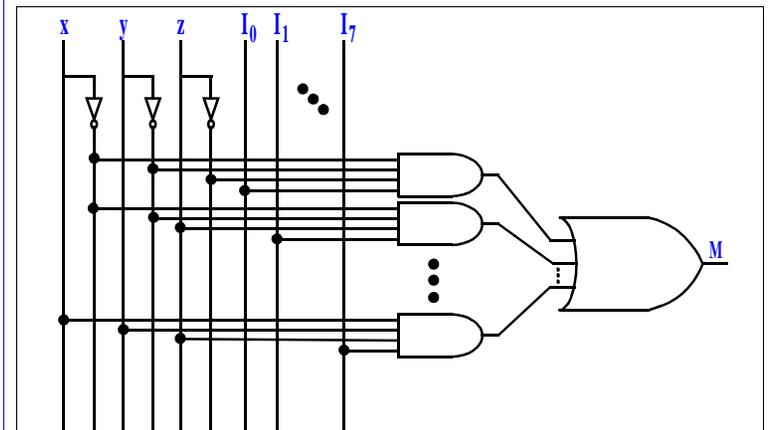
$$M = x'y'z'I_0 + x'y'zI_1 + x'yz'I_2 + x'yzI_3 + xy'z'I_4 + xy'zI_5 + xyz'I_6 + xyzI_7$$
