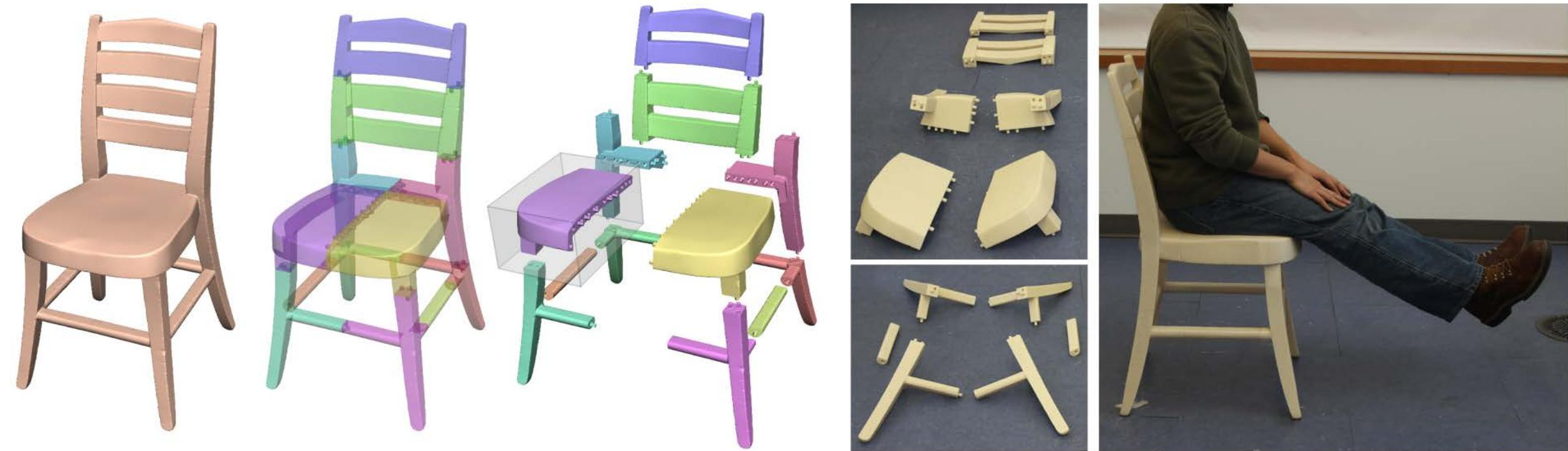
Chopper: Partitioning models into 3D-printable parts [2012]
