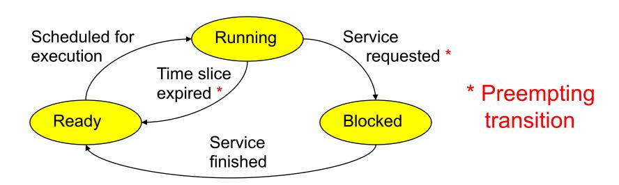
Scheduled for execution: OS selects some process from ready set and assigns CPU to it Time slice expired: OS moves running process to ready set because process consumed its fair share of CPU time Service requested: OS moves running process to blocked set because it requested a (time consuming) system service (often I/O) Service finished: OS moves blocked process to ready set because the requested service finished
