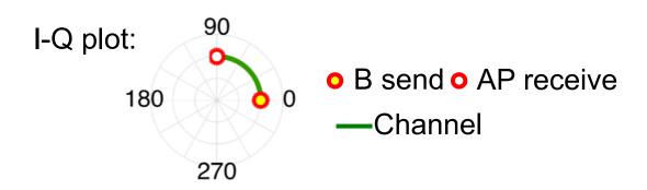
AP can estimate the channel, so can decode User B's signal (o)
