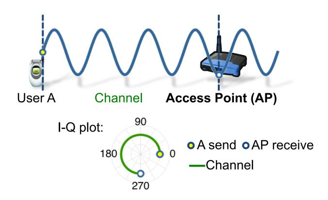
AP can estimate the channel, so can decode User A's signal (o)
