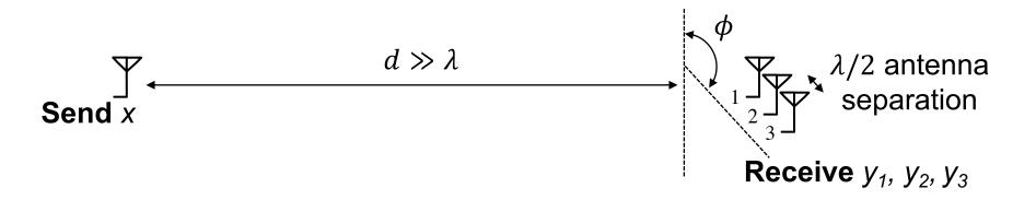
• **Vector notation** for the system:  $\begin{vmatrix} y_1 \\ y_2 \\ y_3 \end{vmatrix} = \vec{y} = \vec{h}x + \vec{w}$
