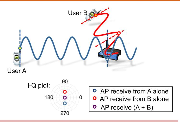
One received signal (o), two sent (o,o), so AP can't decode
