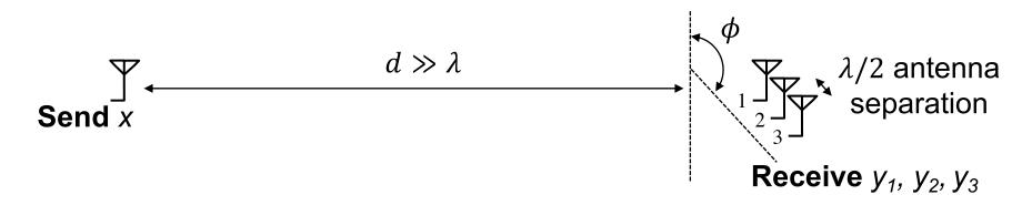
• Maximal ratio combining "projects" the received signals  $\vec{y}$  onto the receive spatial signature:
