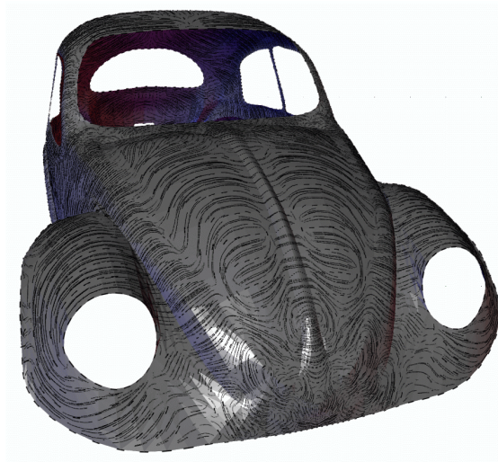
Figure 6.5: Lines of curvature. Lines of curvature are superimposed on a flat shaded image of a VW Beetle model.
