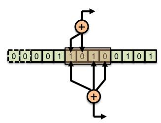
So, d<sub>min</sub> = minimum distance between 000...000 codeword and codeword with fewest 1s
