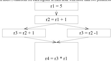
Can insert  $\phi$ -functions for each register at each node with more than two predecessors.
