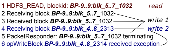
Figure 4: Part of an HDFS log. Request identifiers are shown in bold. Note that the timestamp of each message is not shown.
