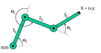
b) True or False: the position X at the end of the arm on the right is uniquely determined by the angles ( $\Theta_1$ ,  $\Theta_2$ , and  $\Theta_3$ ) and lengths ( $l_1$ ,  $l_2$ , and  $l_3$ ), assuming the base point on the left is fixed at (0,0). Please explain your answer. (True or False and one sentence)
