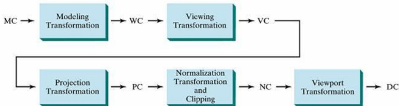
General three-dimensional transformation pipeline, from modeling coordinates to world coordinates to viewing coordinates to projection coordinates to normalized coordinates and, ultimately, to device coordinates.
