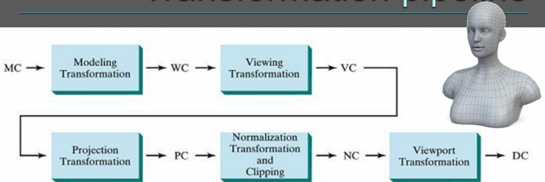
General three-dimensional transformation pipeline, from modeling coordinates to world coordinates to viewing coordinates to projection coordinates to normalized coordinates and, ultimately, to device coordinates.
