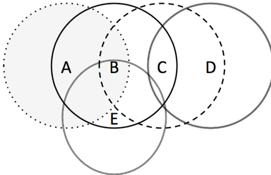
Consider the wireless topology above, comprised of 5 nodes. A (shown in the dotted, shaded circle), B, C, and D all have equi-sized transmission ranges, while E has a smaller range. Assume that if the transmissions of two nodes' will interfere at a location if and only if they transmit at the same time and their transmission areas overlap. In these problems, assume that losses only occur due to collisions.
