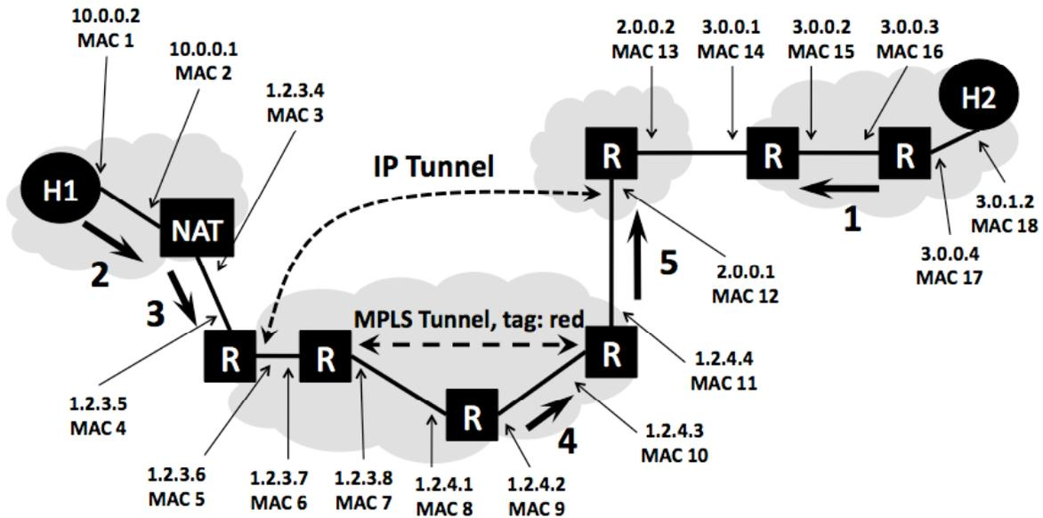
The above figure shows a network topology connecting two LANs. The LAN on the left uses a NAT to connect to the Internet and includes a client host H1. The LAN on the right includes a webserver H2. Packets between the two LANs are routed along the path shown by a heavy dark lines, which includes both an IP tunnel and an MPLS tunnel. All packets which traverse the path use both tunnels. The various network interfaces have IP and MAC addresses as shown.
