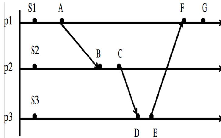
Processes 1, 2, 3 are using a logical clock to keep a consistent time. The horizontal arrow represents physical time and the crossing arrow represents a message being passed. Each point on the horizontal lines is an event.
