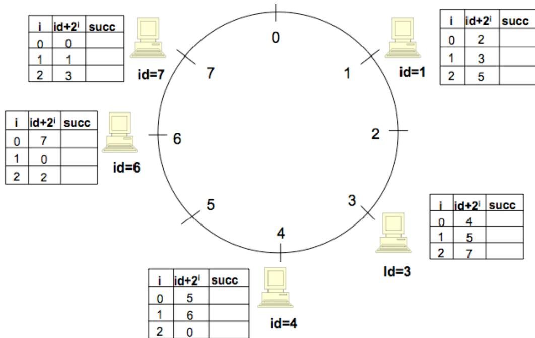
Consider the above illustration of a Chord DHT, comprised of only 5 nodes. We show the finger tables for each node (i.e., the particular id distribution from which a node's routing table neighbors should be drawn), but we don't actually yet fill in the routing tables. Each node may be storing some items according to the Chord assignment rule (remember that Chord assigns keys to nodes in the same way as consistent hashing does, i.e., a successor mod N relationship).
