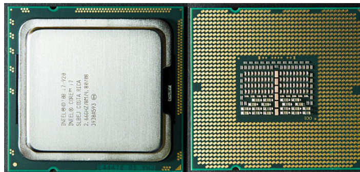
Intel Core i7 microprocessor (around 781 million transistors)
