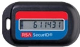
Figure 1: RSA SecurID Device.
