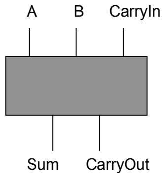
A circuit to compute a single column of an addition is called a 1-bit adder.
