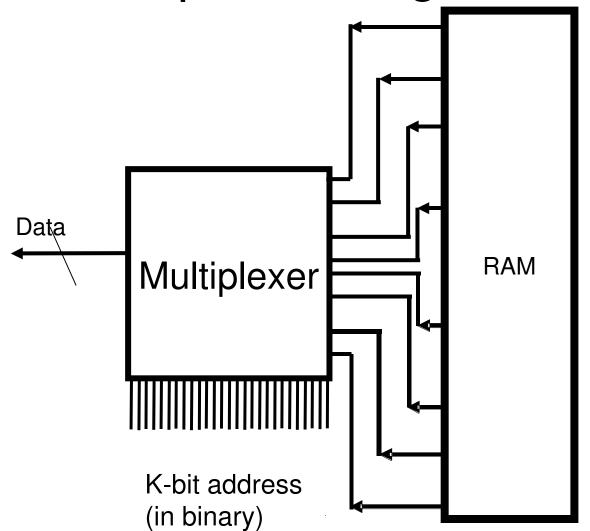
The multiplexer is connected to all cells in the RAM; selects the appropriate cell based upon the k-bit address (simple combinational circuit; see logic handout)
