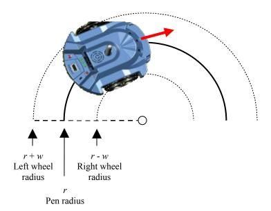
Measure w (half the distance between the wheels). Assume the left motor speed is 100% and solve the
