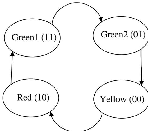
1. Fill in the state transition table of this FSM. The first row is filled out for you. CurrentState1 and CurrentState2 are the two bits of the current state. NextState1 and NextState2 are the two bits of the next state. The output bits are the signals that turn the three LEDs on/off.
