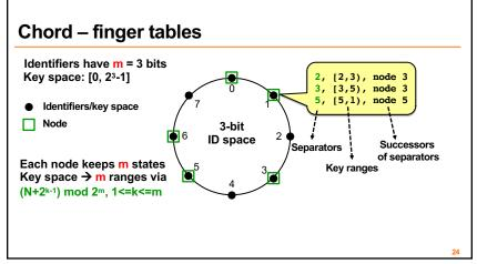
**Chord – finger tables** Identifiers have m = 3 bits 1, [1,2), node 1 Key space: [0, 23-1] 2, [2,4), node 3 4, [4,0), node 5 Identifiers/key space 2, [2,3), node 3 Node ' Node 3-bit 3, [3,5), node 3 5, [5,1), node 5 ID space Each node keeps m states Key space → m ranges via 4, [4,5), node 5 (N+2k-1) mod 2m, 1<=k<=m [5,7), node 5 7, [7,3), node 0 O(logN) messages Look up key 1 and hops!
