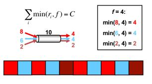
• Associate a weight  $w_i$  with each flow i• If link congested, compute f such that  $\sum_{i} \min(r_i, f \times w_i) = C$   $(w_1 = 3)$   $(w_2 = 1)$   $(w_3 = 1)$   $w_3 = 1$   $w_3 = 1$   $w_4 = 3$   $w_4 = 3$  w
