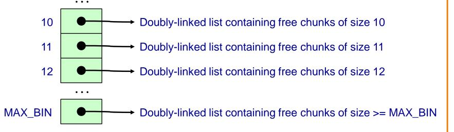
Use an array; each element is a **bin** Each bin is a doubly-linked list of free chunks As in previous implementation bin[i] contains free chunks of size i Exception: Final bin contains chunks of size MAX\_BIN **or larger**
