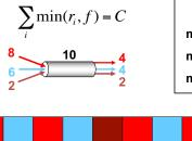
f = 4: min(8, 4) = 4 min(6, 4) = 4 min(2, 4) = 2 • Associate a weight  $w_i$  with each flow i• If link congested, compute f such that  $\sum_{i} \min(r_i, f \times w_i) = C$   $\max_{i} (w_i = 3) \quad 8 \quad 10 \quad 6 \quad \min(8, 2^*3) = 6 \quad \min(6, 2^*1) = 2 \quad \min(2, 2^*1) = 2$
