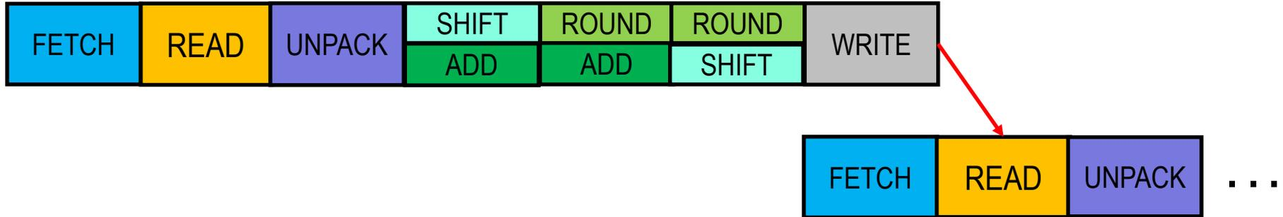
Register bypassing / operand forwarding: extra HW to communicate data directly between FU's
