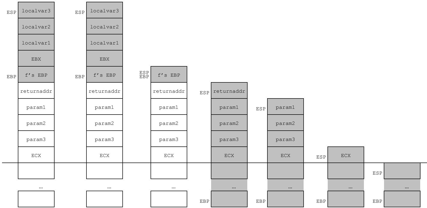
(6) g uses parameters and local variables to compute a return value, and moves that value to EAX:
