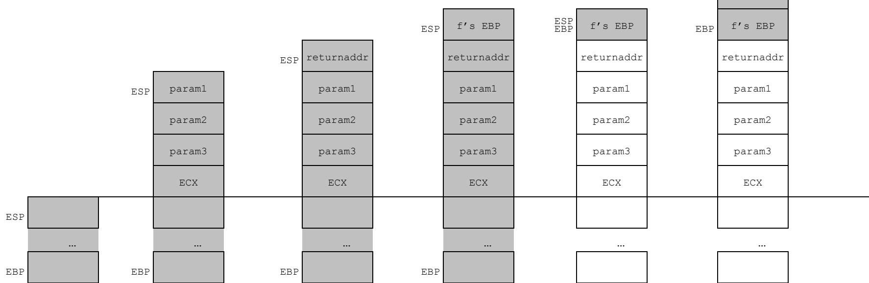
(1) If necessary, f pushes EAX, ECX, EDX, and parameters:
