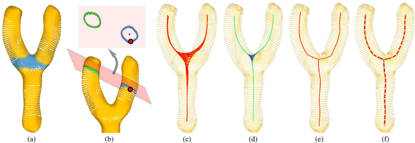
**Figure 5:** Overview of our algorithm. (a) Input point cloud with a joint (blue). (b) Optimal cutting plane and relevant neighborhood points (blue) anchored at a point cloud sample (red particle). (c) Skeletal cloud after ROSA and joint recovery. (d) After thinning with branch (green) and joint (blue) identification. (e) After re-centering, still a skeletal cloud. (f) The final 1D curve skeleton.
