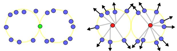
**Figure 4:** Orientation information compensates for missing data. Left: With missing samples from two touch circles and no normals, the computed centroid (green dot) leads to a wrong interpretation of the data. Right: Sample normals reveal two clusters, leading to two ROSA points (red dots). The correct shape can be inferred.
