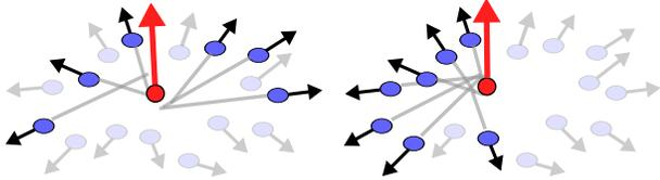
**Figure 3:** Stability of ROSA point position and orientation with more than half of the points missing.
