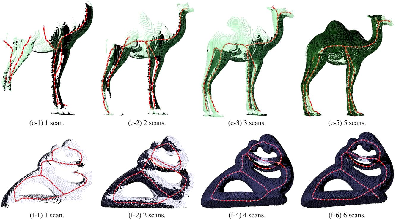
**Figure 9:** Curve skeletons extracted as virtual scans are removed. Here two scans are sufficient to extract a complete skeleton, where about 40% of the points for the fertility model and about 55% of the points for the camel model are missing.
