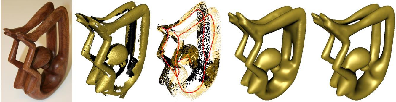
**Figure 1:** From a raw scan with significant missing data, our algorithm extracts a complete curve skeleton, shown in the middle. RBF surface reconstruction infers the wrong surface topology from the original input, while succeeding with the assistance of the curve skeleton.
