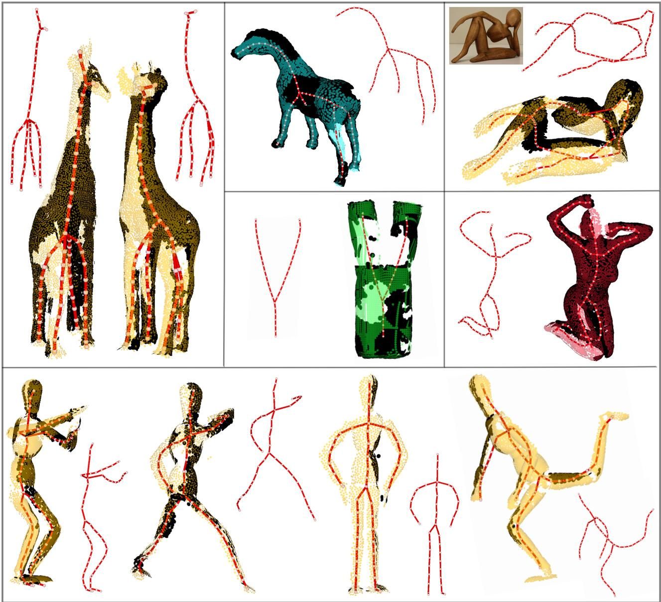
**Figure 10:** A gallery of curve skeleton extraction results. Except for the synthetic “fork” model (green) and the horse, whose missing data are simulated via the virtual scanner, all input come from raw scanned data.
