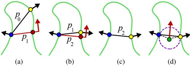
**Figure 6:** 2D illustration of iterative ROSA construction and connection to medial axis. (a-c) Cutting plane anchored at blue sample goes from  $p_0$  to  $p_2$  and converges. During iteration, the normal of the next cutting plane (red) makes the same angle with those normals (black) at the boundary, corresponding to the current cutting plane. (d) When converging, ROSA point (green) is the intersection between two boundary normals and lies on the medial axis.
