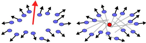
**Figure 2:** ROSA definition for a set of oriented points in 3D. Left: Optimal direction (red arrow) minimizes sum of angular variations with the surrounding normals. Right: Optimal point (red dot) minimizes sum of projected distances to the normal extensions.
