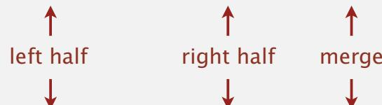
$$A(N) \leq A(\lfloor N/2 \rfloor) + A(\lceil N/2 \rceil) + 6N \text{ for } N > 1, \text{ with } A(1) = 0.$$
