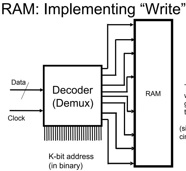
The decoder selects which cell in the RAM gets its "Write" input toggled
