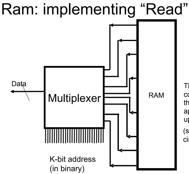
The multiplexer is connected to all cells in the RAM; selects the appropriate cell based upon the k-bit address
