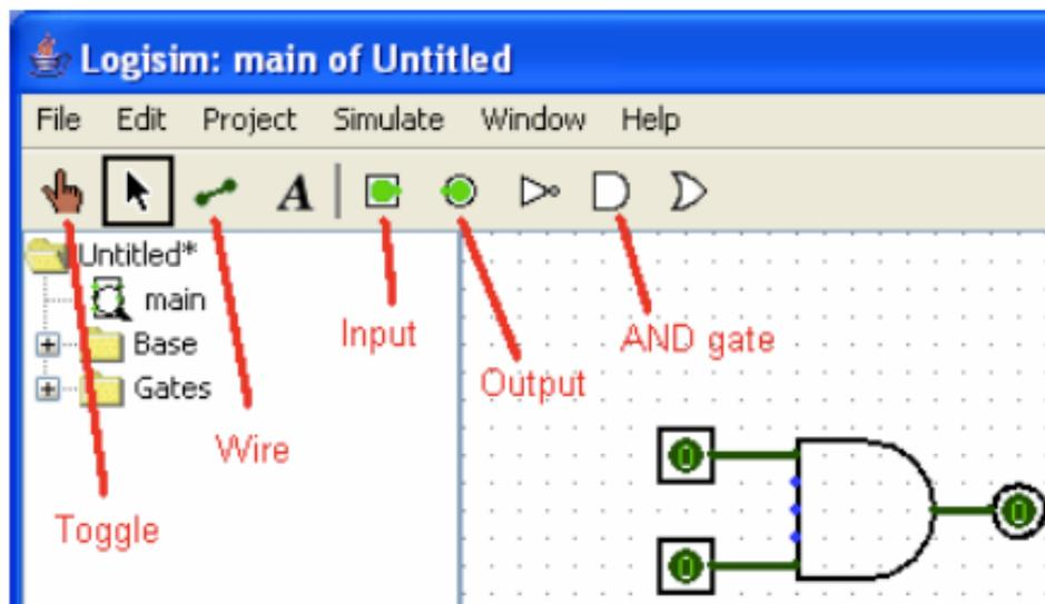
2. Select the AND gate from the toolbar (see figure above), and place the gate anywhere in the dotted field.
