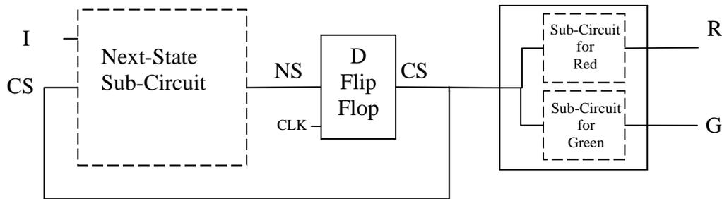
After making this change, every dashed box (i.e. every sub-circuit that we still need to design) has exactly one output. This is the easiest form to work with.
