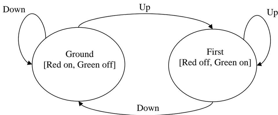
In this diagram, the bubbles represent the states, and the arrows represent state transitions. The arrow labels indicate the input value corresponding to the transition. For instance, when the elevator is in the Ground state, and the input is Up, the next state is First. The information in the brackets indicates the output values for the lights in each state.
