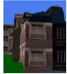
A: Deformation by the impostor representation. A meshed impostor is created without including in the mesh the top-left corner of the front building. This region appears very deformed in the impostor.
