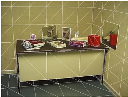
Figure 2: Example of a real image with the superposition of its 3D reconstructed geometrical model (in white)
