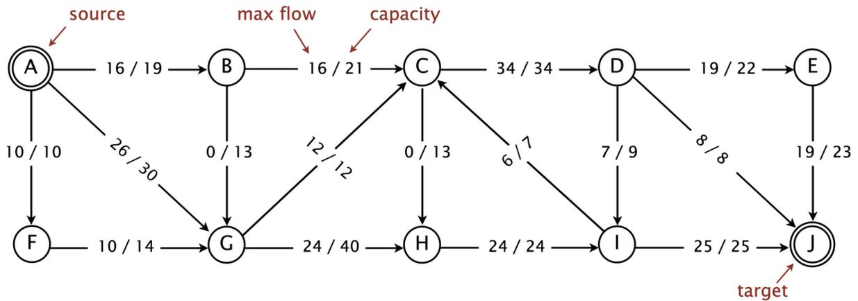
What is the value of  $f$ ? Compute the *capacity* of the cut  $\{A, B, C\}$  and the net *flow* across this cut.
