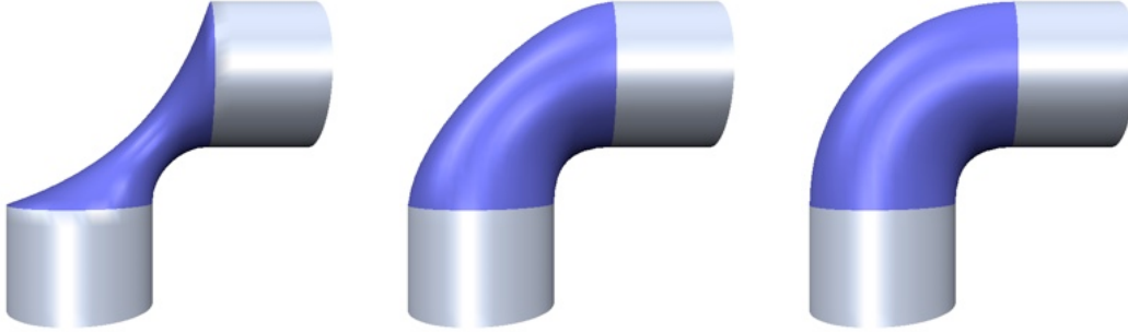
Figure 2.1: This figure shows three examples of fair surfaces, which define a blend between two cylinders. On the left there is a membrane surface which minimizes the surface area. In the center, a thin-plate surface which minimizes curvature. On the right there is a surface which minimizes the variation of mean curvature.
