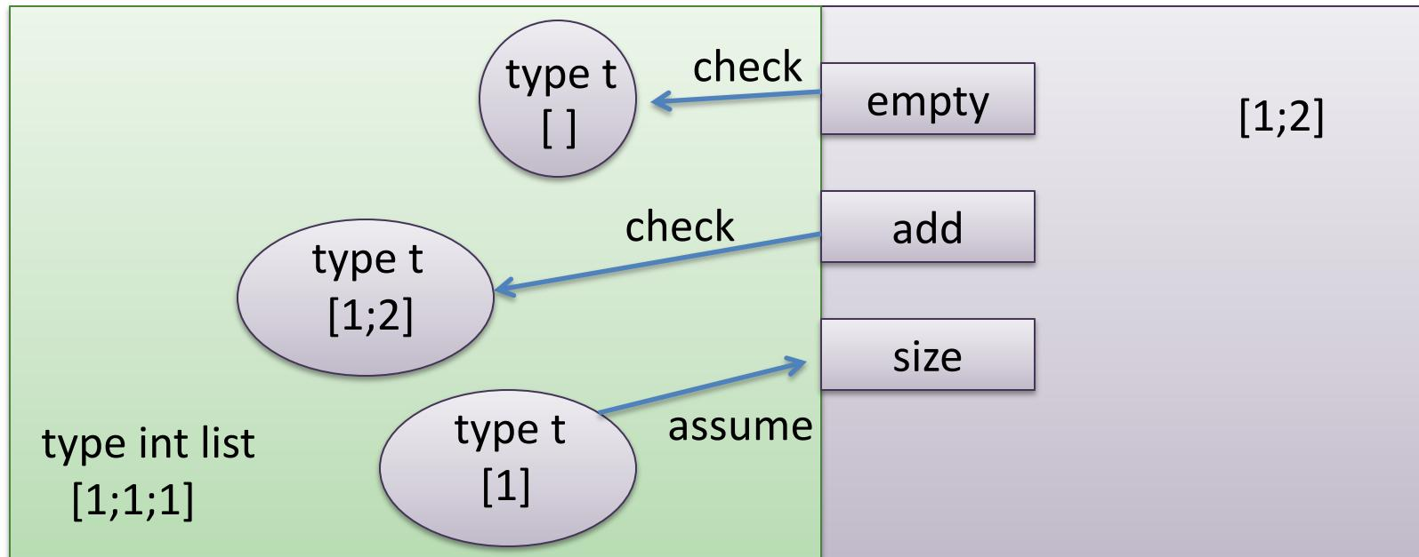
*When debugging*, we can check our invariant each time we construct a value of abstract type. We then get to assume the invariant on input to the module.
