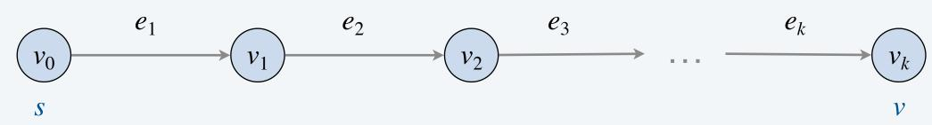
**Corollary.** Bellman–Ford computes shortest path distances. **Pf.** [apply Proposition to a shortest path from s to v]
