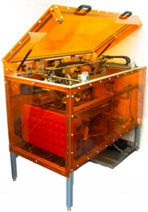
Multifab: A machine vision assisted platform for multi-material 3d printing [2015]
