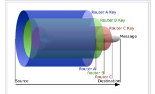
In this example onion, the source of the data sends the onion to Router A, which removes a layer of encryption to learn only where to send it next and where it came from (though it does not know if the sender is the origin or just another node). Router A sends it to Router B, which decrypts another layer to learn its next destination. Router B sends it to Router C, which removes the final layer of encryption and transmits the original message to its destination.
