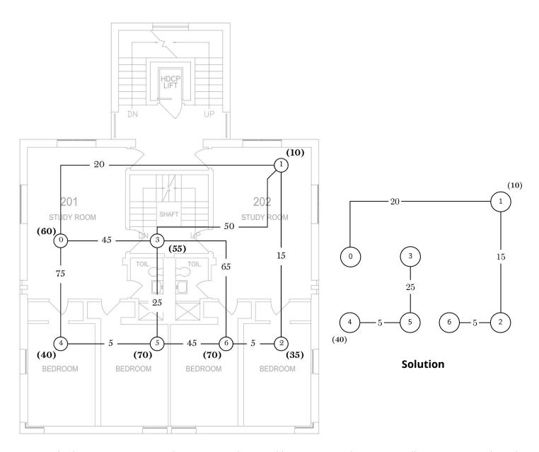
For example, this instance contains 7 dorm rooms and 10 possible connections. The router installation costs are indicated in bold and parentheses; the fiber costs are given on the edges. The optimal solution, which costs 120, installs a router in rooms 1 and 4 (for a cost of 10 + 40) and builds the shown fiber connections.
