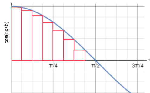
Figure 2.1: Approximation of cosine function using step function.
