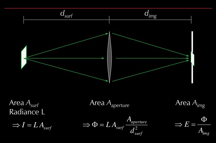
$$I = LA_{surf} \qquad \Phi = LA_{surf} \frac{A_{aperture}}{d_{surf}^2} \qquad E = \frac{\Phi}{A_{img}}$$
