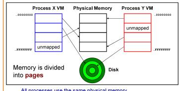
All processes use the same physical memory Hardware and OS provide application pgms with a virtual view of memory, i.e. virtual memory (VM)
