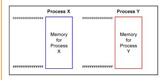
Hardware and OS give each application process the illusion that it is the only process using memory
