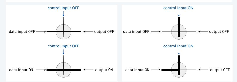
Idealized model of *pass transistors* found in real integrated circuits.
