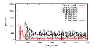
Figure 6: Four TCP-SACK flows and four CUBIC flows over  $40 \mathrm{ms} \ \mathrm{RTT}$
