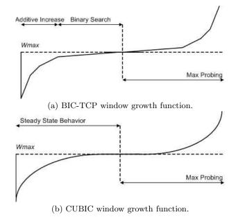
Figure 1: Window growth functions of BIC-TCP and CUBIC.
