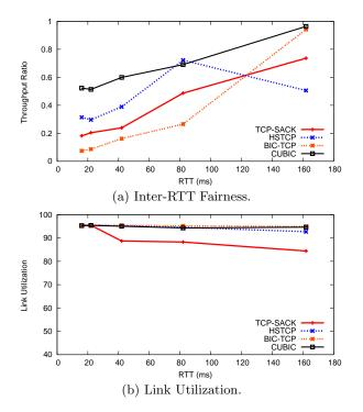
Figure 9: Inter-RTT fairness. The bottleneck bandwidth is set to 400Mbps and 2Mbyte buffer is used. One flow has a fixed RTT of 162ms and the other flow varies its RTT from 16ms to 162ms.
