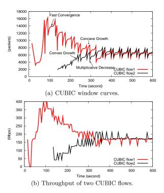
Figure 4: Two CUBIC flows with 246ms RTT.
