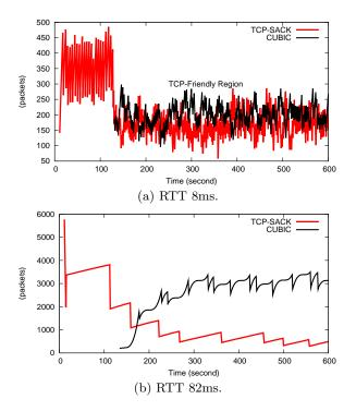
Figure 5: One CUBIC flow and one TCP-SACK flow. Bandwidth is set to 400Mbps.
