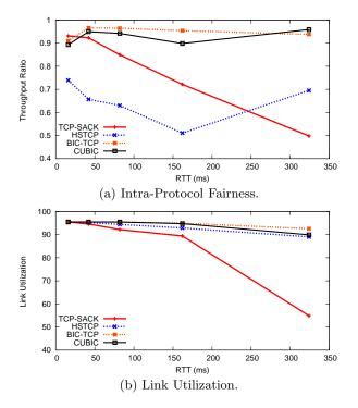
Figure 8: Intra-protocol fairness (a) and link utilization (b). The bottleneck bandwidth is set to 400Mbps and 2Mbyte bottleneck buffer is used. RTT is varied between 16ms and 324ms and two flows have the same RTT.
