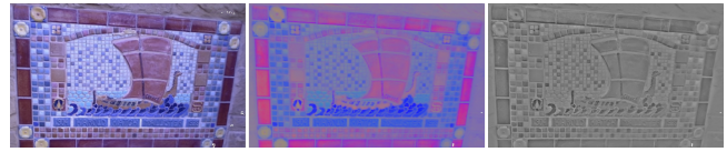
Figure 6: From left to right: fused model color, chromaticity, and estimated per voxel albedo luminance estimate \mathbf{a}(\mathbf{v}) .
