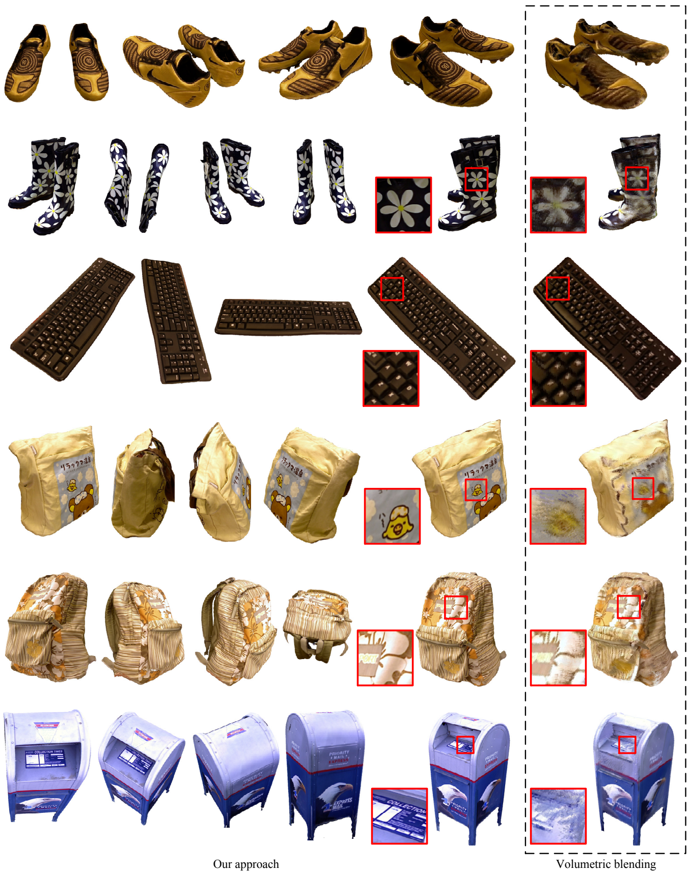
Figure 4: A variety of additional objects reconstructed by the presented approach. For reference, the color maps produced for the same input by the widely used volumetric blending approach as implemented in the state-of-the-art Point Cloud Library are shown on the right.
