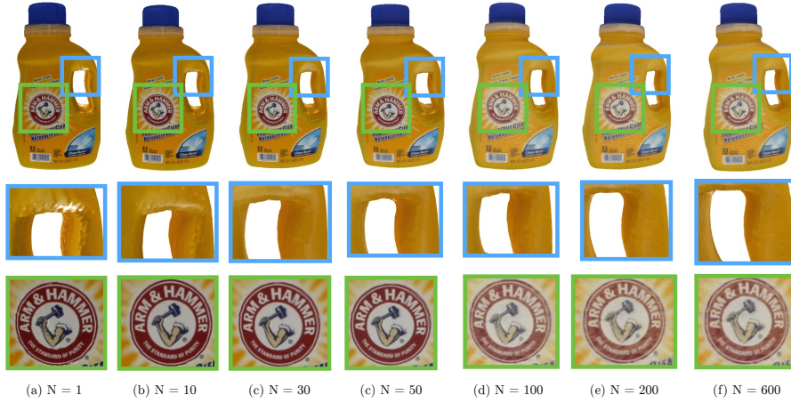
Fig. 3. The effect of N = |V'(\mathbf{p}; t_{\mathbf{p}})| on the sharpness of textured regions and the smoothness of non-textured regions: smaller (larger) N yield sharper (faded) textures, but blotchy (smooth) non-textured regions. When N = 1 , we observe white regions on the detergent handle because these colors incorrectly bleed onto the white turntable background in the best viewing image; larger N rectify this problem.
