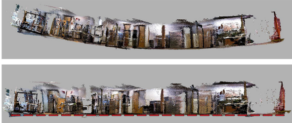
Figure 2: Fitting and enforcing a structural model comprising planes with long-range constraints can yield more accurate global registration. The top image shows our registration result without detecting and enforcing a structural model, and the bottom one shows our result. The horizontal red line depicts the planar proxy found in the later iterations of our algorithm that guides the optimization to the correct solution.
