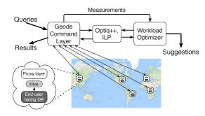
Figure 3: Geode architecture
