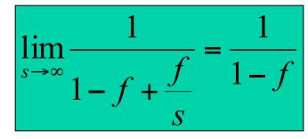
where f is fraction optimized, s is speedup of that fraction
